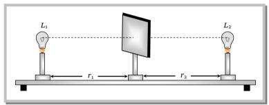
Two sources of luminous intensity  $L_1$ , and  $L_2$  are placed at distances  $r_1$  and  $r_2$  from the screen so that their flux are perpendicular to the screen. The distance  $r_1$  and  $r_2$  are adjusted till  $I_1 = I_2$ .
